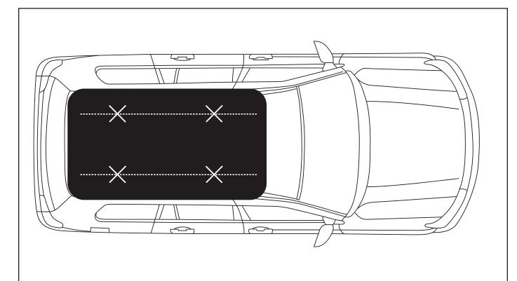
5. The RTT should have 4 spaced, strong points of contact on the roof rack. Take the vehicle for a low speed, short drive. Afterwards, check all the bolts are secure. Tighten if required.
